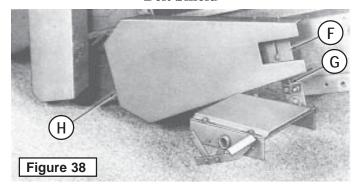
Fig. 38 - Attach back guard "F" to belt shield using (4) #14 x 1/2" tapping screws. Attach mounting bracket "G" to guard "F" using a 3/8" x 1" machine bolt with flat washer next to slotted hole. Attach bracket "G" to bolt found in engine mounting. Attach lower end of shield to boot at "H" using (2) #14 x 1/2" tapping screws. Tighten all bolts.
