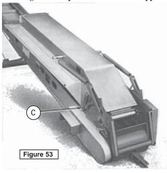
Fig. 53 The illustration above shows the hopper in the storage or transport position. Locate pins to second hole from bottom (over stop arm) at "C" (both sides) when this is done.
