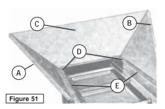
Fig. 55 - Attach hopper sides "A" and "B" to hopper end "C" using 3/16" x 1/2" machine screws.
