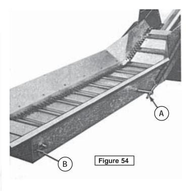
Fig. 54 - To adjust the lift springs, adjust nuts on eyebolts "A" to the point where the hopper merely rest on the ground. To adjust the conveyor, adjust nut on bolts "B" (both sides) so when lifting the conveyor in the center between slides and sprockets, it can be lifted from 2-1/2" to 3".
