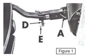
Fig. 1 - Before hitching elevator to tractor, support pin "A" must be installed as shown. Make sure to use pin clip "E" in hitch pin "D" prior to transporting.
