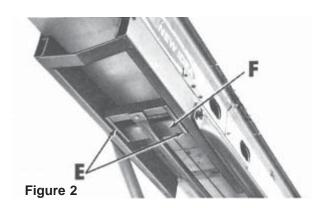
Fig. 2 - Never transport the elevator unless the transport lock assembly "E" is engaged with the boom clevis "F".
