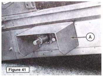
Fig. 41 -Attach PTO shield "A" to bolts found in flangettes. Note: This shield is used for PTO drive elevator only, regardless to which side it is to be driven from.
