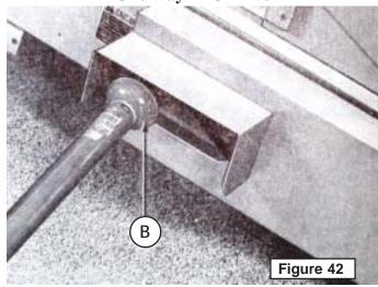
Fig. 42 -Attach PTO assembly to drive shaft at "B" using a 5/16" x 2-1/2" machine bolt.
